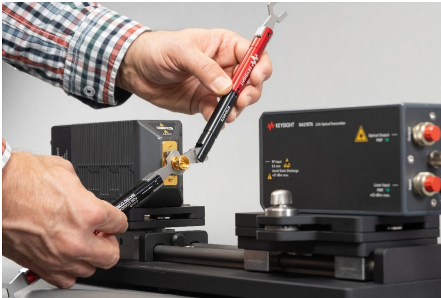
Figure 4. Preparing frequency extender and optical transmitter to connect, using the N4378FA mechanical fixture
